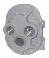
Model GP-PTO is a rear-ported, Power Take Off gear pump constructed with cast iron end plates and an aluminum center section. This pump offers a 9.76 in<sup>3</sup>/rev (160 cm<sup>3</sup>/rev) displacement and higher flows at reduced engine rpm as compared to other PTO pumps. Standard drive is 1 <sup>3</sup>/8" diameter 21-tooth female spline.
